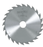
TCT saw blade 185 x 1.4/2.4 x 20 mm, ATB, 24 teeth, for universal use with wood
