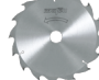
TCT saw blade 185 x 1.4/2.4 x 20 mm, ATB, 16 teeth, for ripping in wood
